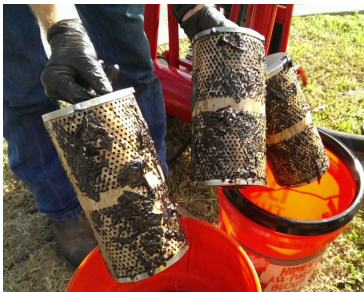
Dirty fuel filters after polishing!
