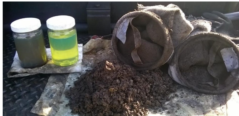
Before and after fuel samples alongside the sock filters used in this filtering process with the sediment filtered out of the fuel.
